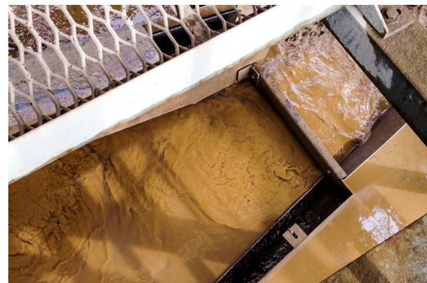
LOAD ZONE BAFFLE SETTLES FINES
