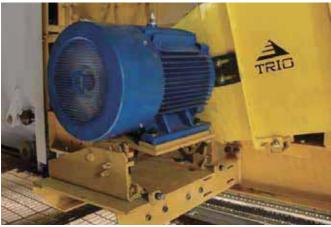
TTH Series Screens generate power via three timed shafts with eccentric counterweights. The combination of the three shafts provide an oval stroke with adjustable amplitude, speed and operating angle, determined by application.
