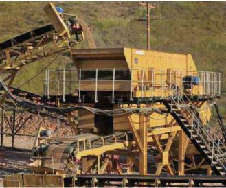
The applications for Horizontal screens include: when a slower material travel rate is required such as when fine sized screening with a large percentage of near size product, or when low head room is critical, and also fine screening of dry products or wet washing.
