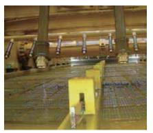
Screen decks can accommodate all media types, wire cloth, urethane, and rubber. Flat decks are available.
