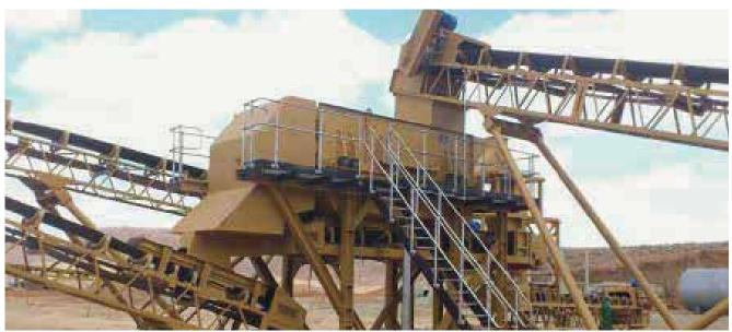
TRIO modular structures incorporate heavy duty structural steel weldments using bolted connections. Safe and accessible work areas are built with grated stairways and work platforms equipped with hand, knee and toe rails providing labor saving installation.
