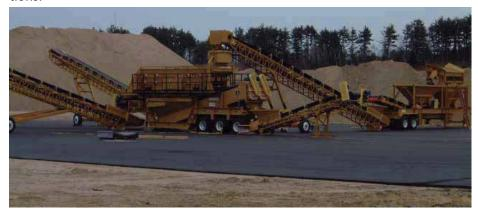
TRIO's portable plants boost efficiency; maximizes setup flexibility and provide better access to material resources.
