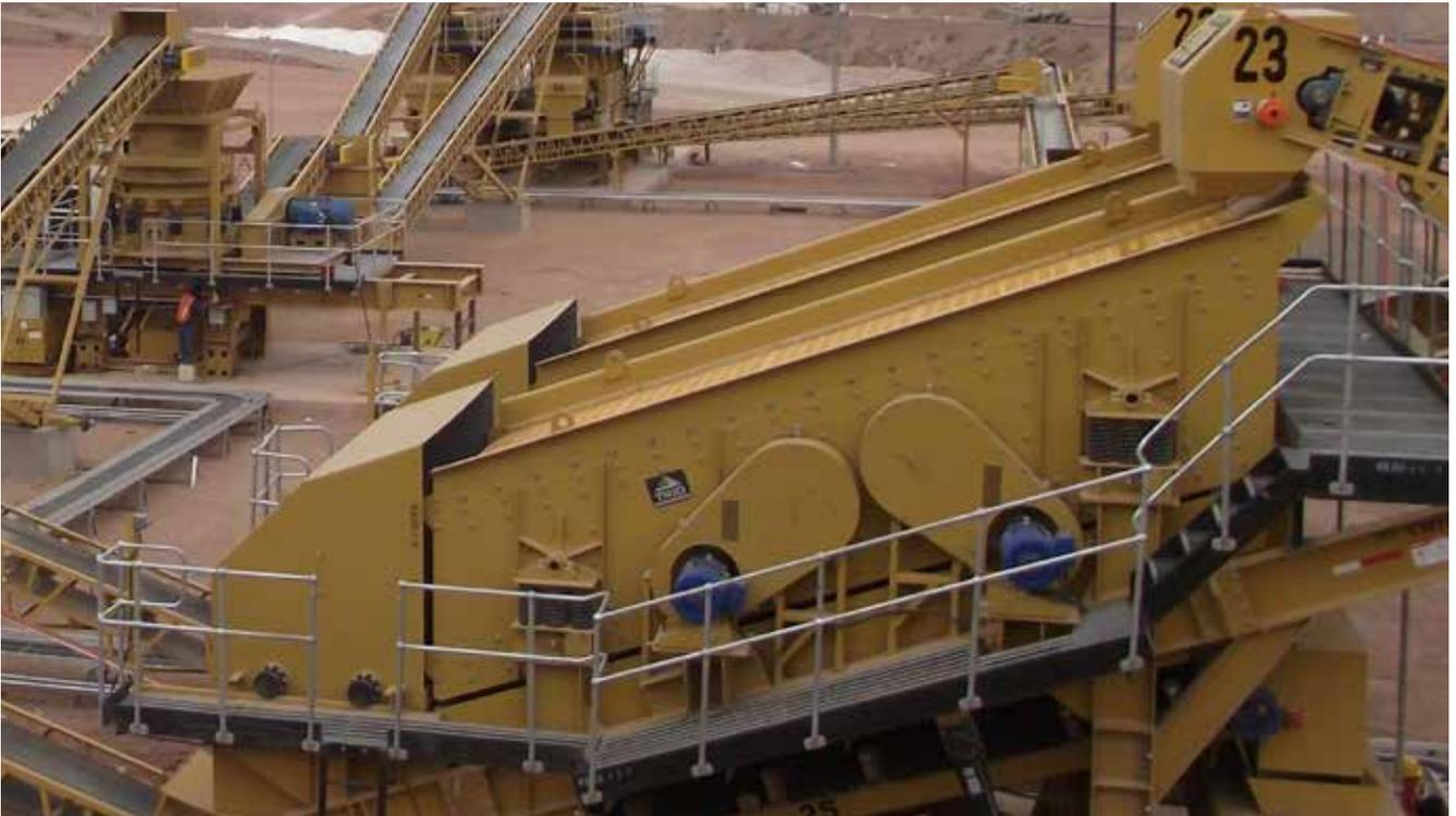
The TIO Series screens are designed for continuous operation in the most demanding applications and have a wide range of applications in both wet and dry operating scenarios with a feed acceptance size of 8". The operating inclination can be varied from 15 to 20 degrees depending on the velocity required to stratify the material.
