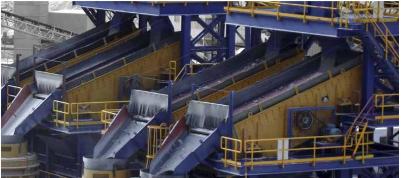
All components mounted to the screen side panels are attached with Huck bolts. The vibrating units are attached with threaded bolts for easy servicing. No welding is used; this process insures rigidity and structural integrity and eliminates stress fatigue in the screen body insuring a long productive service life.
