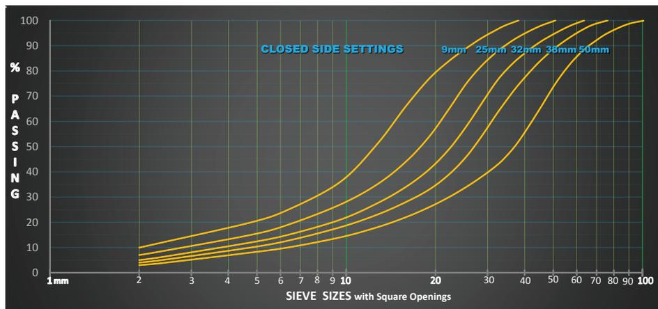
\* Data collected when material compressive strength from 110 to 140 Mpa, build specific weight at 1.6 metric ton/m<sup>3</sup>, humidity <=4%, with appropriate feeding material gradation. Please contact us for detailed info.
