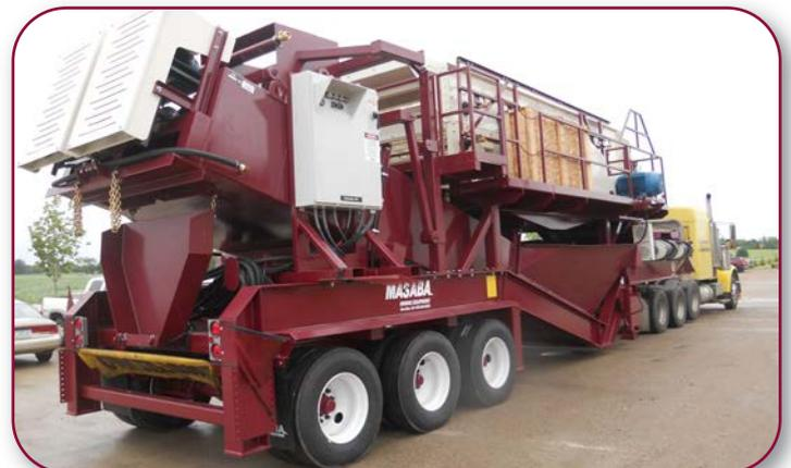
Portable Wash Plant with Cedarapids 6x20TD screen over MASABA 36"x 25' twin screws
