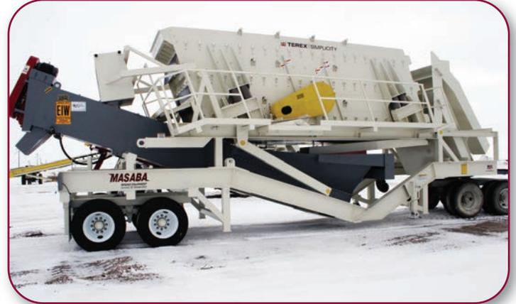
Portable Wash Plant with Simplicity 6x16TD incline screen over Eagle Single 36"x 25' screw
