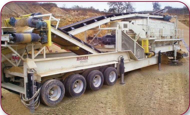
Portable Cone Plant with Cedarapids MVP 380 cone, Cedarapids 6x20TD screen, (1) 60" under screen conveyor, (1) 18" top cross conveyor, (1) 24" bottom cross conveyor, (1) 42" feed conveyor, (1) 36" under crusher conveyor, and (1) 36" rear cross conveyor, and **MASABA** "Brute" run-on jacks
