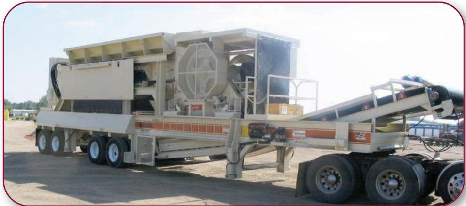
Portable Crushing Plant with Metso C106 Jaw, 58"x20' vibrating grizzly feeder and 48" front discharge conveyor
