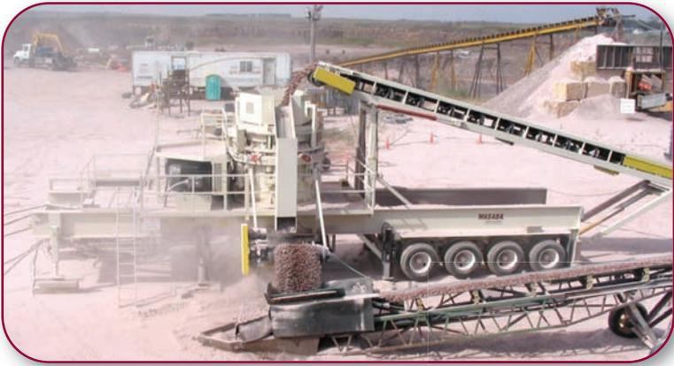
Portable Open Circuit Cone Plant with Cedarapids MVP550 cone, dual 250HP drive, 48" hydraulically folding side discharge conveyor and hydraulically adjustable 42" feed conveyor, and **MASABA** "Brute" run-on jacks
