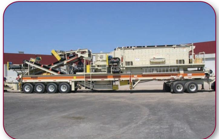
Portable Closed Circuit Crushing Plant with Metso HP300 cone and Metso 6x20TD Screen, (1) 60" under screen conveyor, (1) 18" top cross conveyor, (1) 24" bottom cross conveyor, (1) 42" feed conveyor with hydraulic fold, (1) 42" under crusher conveyor, (1) 36" cross conveyor and (6) leveling jacks
