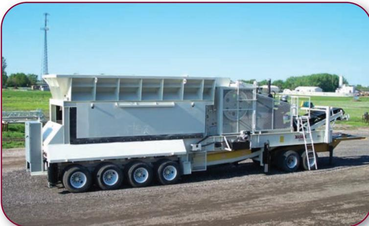
Portable Crushing Plant with Cedarapids 3042, 58"x20' vibrating grizzly feeder and 48" front discharge conveyor
