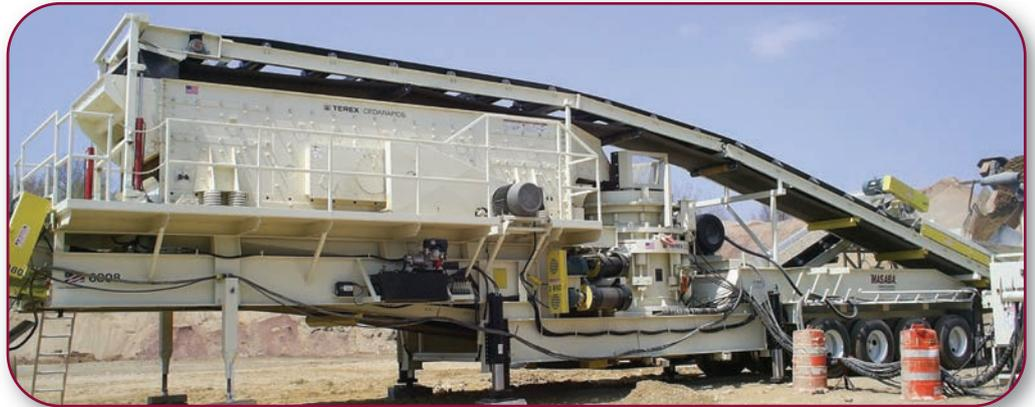
Portable Closed Circuit Crushing Plant with Cedarapids MVP 280 cone, Cedarapids 6x20TD Screen, (1) 60" under screen conveyor, (1) 18" top cross conveyor, (1) 24" bottom cross conveyor, (1) 42" feed conveyor, (1) 36" under crusher conveyor, (1) 36" rear cross conveyor, and **MASABA** "Brute" run-on jacks
