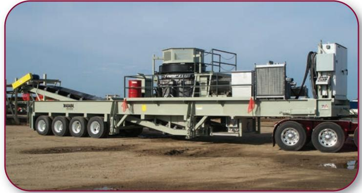
Portable Crushing Plant with Raptor Excel 400 cone, (1) 42" discharge conveyor
