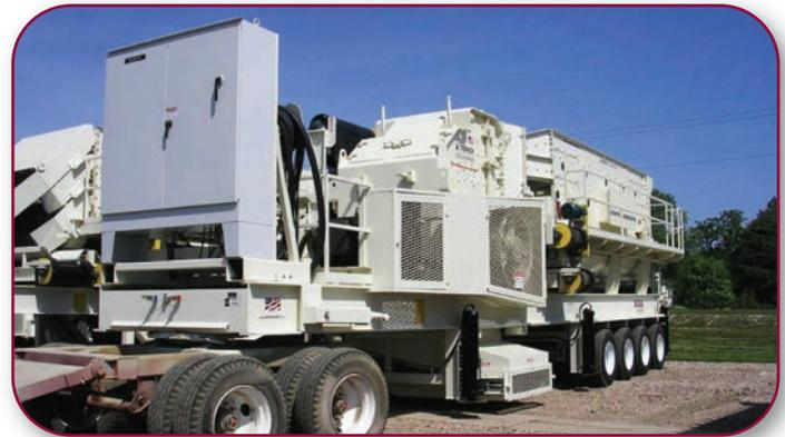
Portable Crushing Plant with Cedarapids 5048 secondary impactor, Cedarapids 6x20TD screen, 48" fold-up side discharge conveyor, (2) 24" side discharge conveyors, and **MASABA** "Brute" run-on jacks
